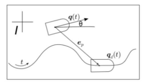
The tracking error vector e is conveniently expressed in terms of its projections on the rotated reference frame of the robot wrt to the inertial frame. In this way the positional part of the error is the Cartesian component of the error expressed in a reference frame aligned with the current orientation of the robot:
