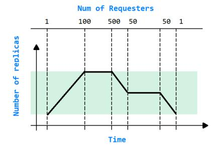
Figure 2: Linear Replication Policy with an upper-bound
