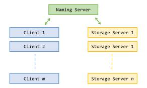
Figure 1: Architecture of *FileStack (Project 1)*
