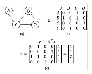
Figure 1: Graph (a) Logical representation (b) Adjacency matrix (c) In-degree calculation as SPMV GT  $\mathbf{x} = \mathbf{y}$ . Vector  $\mathbf{x}$  is all ones. The output vector  $\mathbf{y}$  indicates the number of incoming edges for each vertex.
