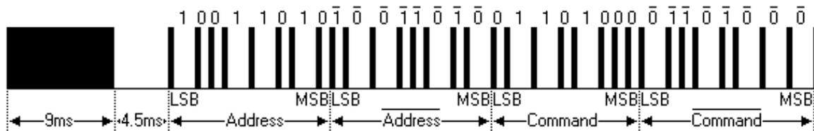
A command is transmitted only once, even when the key on the remote control remains pressed. Every 110ms a repeat code is transmitted for as long as the key remains down. This repeat code is simply a 9000 $\mu$ s LOW pulse followed by a 2250 $\mu$ s HI and a 560 $\mu$ s LOW. In this task, you can ignore (discard) the repeat commands.
