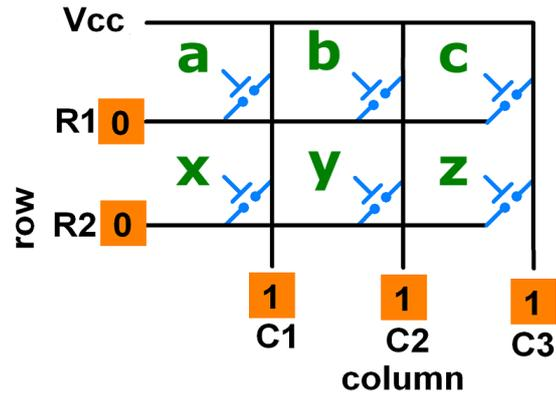
You can assume that the circuit works as follows: when R1 is LOW and button 'a' is pressed, C1 will be LOW, when R2 is LOW and button 'y' is pressed, C2 will be LOW, ...
