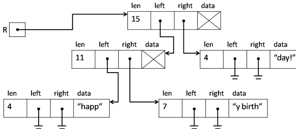
Note that where we indicate Xes in the **data** field, any contents would be allowed and we would still have a valid rope. We can also represent the same structure using a short-hand notation that illustrates the two different types of nodes, leaf nodes and concatenation nodes:
