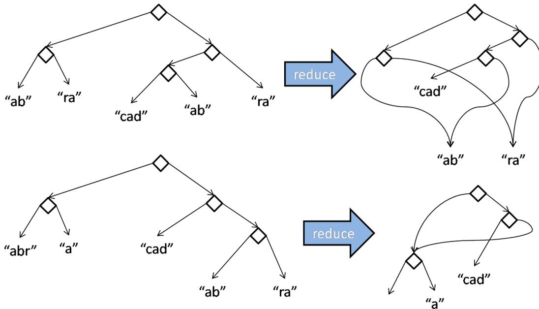
Your memory-reduction procedure will use a hashtable-based dictionary. When given a rope, you should look up that rope in the dictionary to see if an equivalent rope (one representing the same string) already exists. If so, your memory-reduction procedure can just return that already-stored rope in place of the rope you were given.
