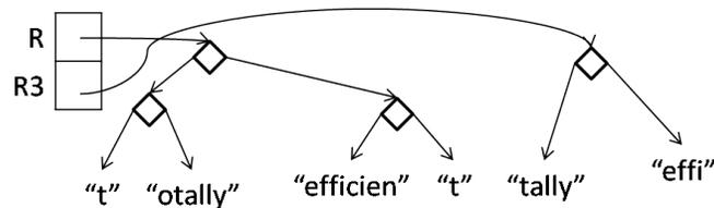
Running `rope_sub(R, 0, 1)` and `rope_sub(R, 7, 16)` should not cause *any* new memory to be allocated, because these substrings are captured by subtrees of the original rope. Running `rope_sub(R, 2, 3)` must return a newly-allocated leaf node containing the string "t".
