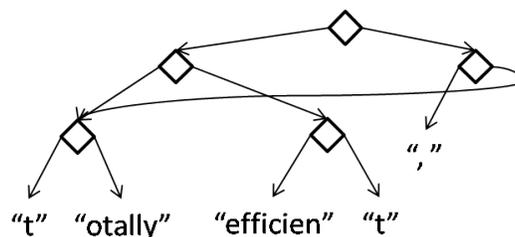
Structure sharing for ropes only works because none of the rope interface functions allow us to modify ropes after they have been created. By sharing structure, we can make very very big strings without allocating much memory, and this is one reason it was necessary to add the precondition checking for overflow to `rope_join`.
