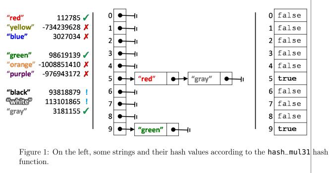
In the middle, a separate-chaining hash table using this hash function, after the insertion of the strings "green", "red", and "gray". Next to them is an indication of whether the Bloom filter (first implementation) returns a true positive ( $\checkmark$ ), a false positive (!), or a (true) negative ( $\checkmark$ ).
