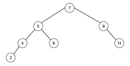
Inserting 1 as in a binary search tree will place it to the left of 2, causing violations at nodes 4, 5 and 7. A (single) right rotation at the lowest of these violations, node 4, fixes it, producing the following tree:
