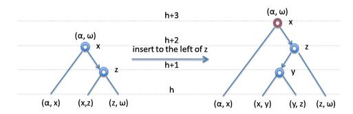
In the situation on the right, the subtrees labeled  $(\alpha, x)$  and  $(z, \omega)$  must have exactly height h, but only one of (x, y) and (y, z) does. In this case, a single left rotation alone will not restore the invariant (see Exercise ??). Instead, we apply a so-called *double rotation*: first a *right* rotation at z, then a *left* rotation at the root labeled x. When we do this we obtain the picture on the right, restoring the height invariant.
