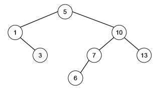
After inserting 4, the height invariant at node 1 is violated.
