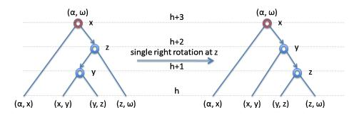
The tree rooted at z has height h+1 since its right subtree has height h and its left subtree has height at most h. The tree rooted at y has height h+2 since its right subtree has height h+1 and its left subtree has height at most h. Note that there could be a violation at y. The tree rooted at x still has height h+3 since its right subtree has height h+2 and its left subtree has height h— there is definitely a violation at x still although it may not be the lowest any more.
