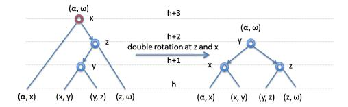
To apply this rotation, the nodes x, y and z must exist. Furthermore, since it is applied at the lowest violation, both the right and left subtree of x are valid AVL trees. Since it fixes the violation, the tree rooted at y is a valid AVL tree. This defines the contracts of rotate\_left\_right.
