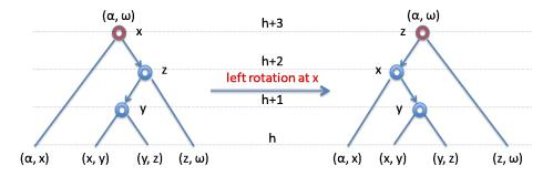
The left subtree of x still has height h since it was not modified. Its right subtree is the original subtree rooted at y, which has height h+1. Therefore the updated tree rooted x has now height h+2, which forces its parent, z, to be the root of a tree of height h+3. Thus, the left subtree of z has height h+2. However, its right subtree still has height h since it was not modified. We have a violation at z.
