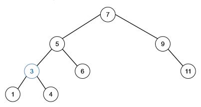
Notice that a single rotation was applied when the new node was initially inserted in an outer subtree of the tree rooted at the lowest violation, while a double rotation was used when the insertion occurred in an inner subtree. This observation applies generally.
