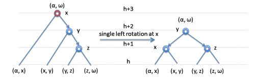
The tree rooted at z is unchanged and therefore its height remains h+1. The tree rooted at x now has height h+1 because its left subtree has height h and its right subtree has height at most h. This makes y the root of two subtrees of height h+1 and therefore the overall tree rooted at y has height h+2.
