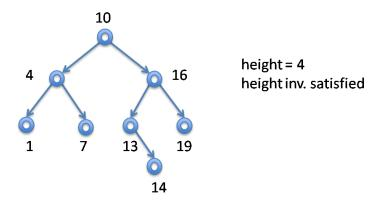
Now the tree has height 4, and one path is longer than the others. However, it is easy to check that at each node, the height of the left and right subtrees still differs only by one. For example, at the node with key 16, the left subtree has height 2 and the right subtree has height 1, which still obeys our height invariant.
