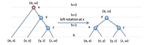
We fix this with a left rotation at x, the result of which is displayed to the right. Because the height of the overall tree is reduced to its original h + 2, no further rotation higher up in the tree will be necessary.
