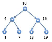
height = 3 height inv. satisfied If we insert a new entry with a key of 14, the insertion algorithm for binary search trees without rebalancing will put it to the right of 13.
