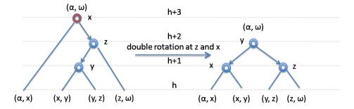
Recall that left subtree of node x and the right subtree of z must have height h, and at least one of the subtrees of y also has height h — the other could have height h-1.
