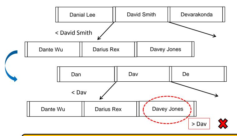
To ensure correct semantics, the <u>largest key value in the left sub-tree</u> and the <u>smallest key value in the right sub-tree</u> must be examined!
