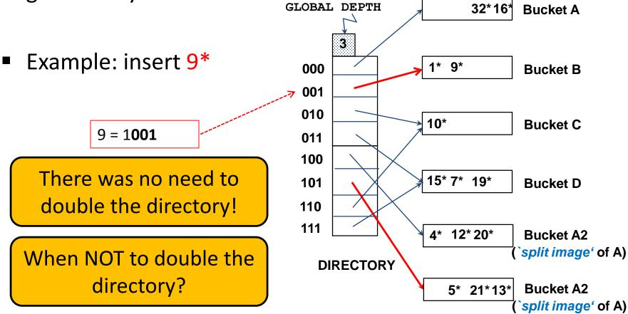
Find the appropriate bucket (as in search), split the bucket if full, double the directory if necessary and insert the local DEPTH
