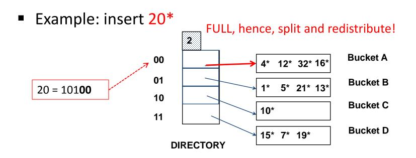
Find the appropriate bucket (as in search), split the bucket if full, double the directory if necessary and insert the given entry
