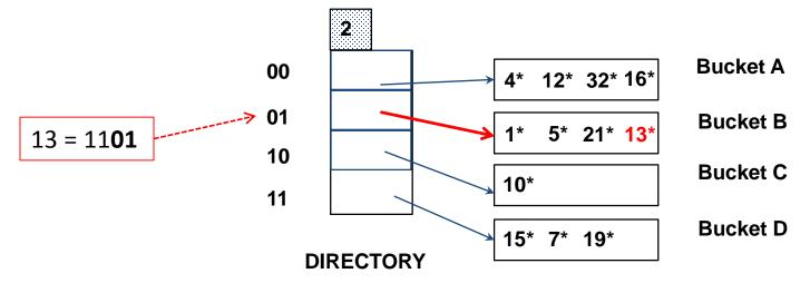
Find the appropriate bucket (as in search), split the bucket if full, double the directory if necessary and insert the given entry
