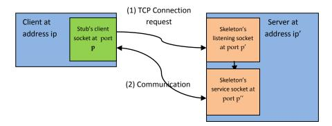
Figure 3: Sockets and Multi-threading.
