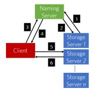
Figure 1: Architecture of FileStack
