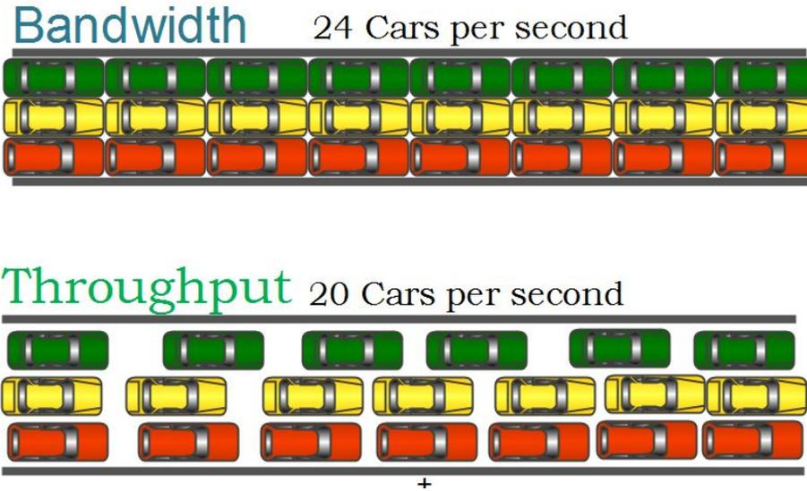
**Fig1.** Difference between throughput and bandwidth
