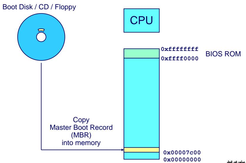
Boot Disk / CD / Floppy **CPU** 0xffffffff **BIOS ROM** 0xffff0000 **BIOS** verifies MBR and jumps to 0x00007c00 0x00007c00
