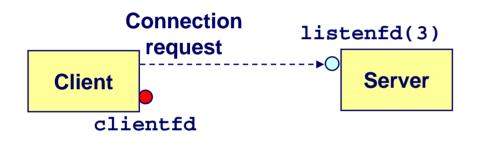
2. Client makes connection request by calling and blocking in connect.
