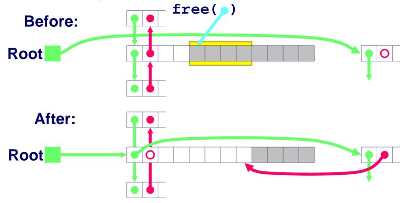
Splice out predecessor block, coalesce both memory blocks and insert the new block at the root of the list
