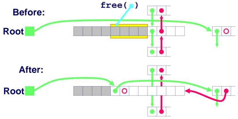
Splice out successor block, coalesce both memory blocks and insert the new block at the root of the list
