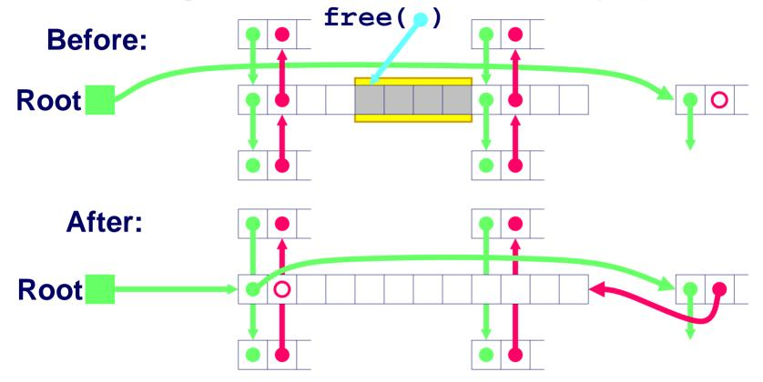
Splice out predecessor and successor blocks, coalesce all 3 memory blocks and insert the new block at the root of the list
