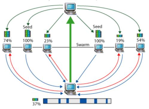
Computer with BitTorrent client software receives and sends multiple pieces of the file simultaneously.
