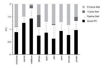
Figure 4. IPC Breakdown for a single 2-issue processor.
