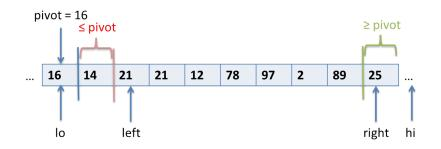
In the next two steps, we proceed by making swaps. First, we decide that the 21 that is currently at *left* can be properly placed to the left of the 25, so we swap it with the element to the left of 25. Then, we have 89 at A[left], and so we can decide this is well-placed to the left of that 21.
