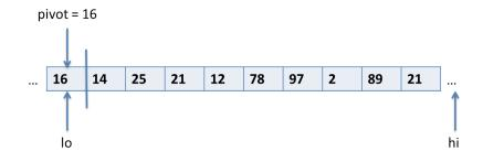
Now the idea is to gradually work towards the middle, accumulating elements less than the pivot on the left and elements greater than the pivot on the right end of the segment (excluding the pivot itself). For this purpose we introduce two indices, *left* and *right*. We start them out as lo + 1 (to avoid the stashed-away pivot) and *hi*.
