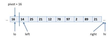
Since 14 < pivot, we can advance the *left* index: this element is in the proper place.
