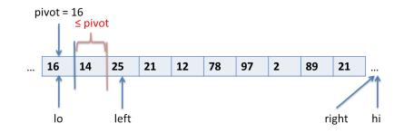
At this point, 25 > pivot, it needs to go on the right side of the array. If we put it on the *extreme* right end of the array, we can then say that it is in its proper place. We swap it into A[right - 1] and decrement the *right* index.
