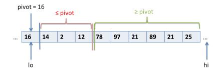
Where do *left* and *right* need to be, according to our invariants? By invariant (1), all elements up to but excluding *left* must be less than or equal to *pivot*. To guarantee we are finished, therefore, the *left* index must address the element 78 at lo + 4. Similarly, invariant (2) states that the pivot must be less than or equal to all elements starting from *right* up to but excluding *hi*. Therefore, *right* must also address the element 78 at lo + 4.
