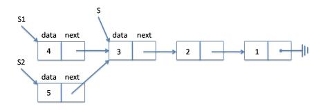
All three stacks share nodes 3, 2 and 1. Observe furthermore that the second call to push operated on S, which remained unchanged after the first call. At this point, a pop on S would result in a fourth stack, say S3, which points to node 2.
